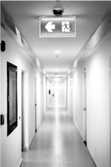
*Emergency lighting plays a very important role in building safety and especially in the evacuation scenario. The emergency lighting system is designed to provide automatic lighting in an emergency situation when the main power supply is interrupted and normal mains lighting is disabled. Emergency lighting systems serve as a lifeline in dangerous situations by reducing panic, providing necessary lighting and directing people in the building to safe exit points.*
